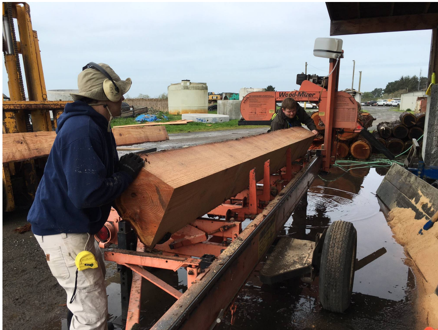
City employees milling blow down logs at Corp yard mill for bench and bridge material.
