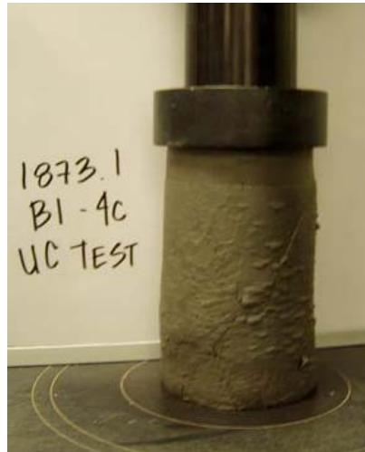
**Unconfined Compression Test Readings**
