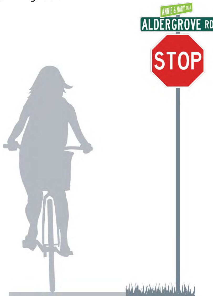
Figure 31: Example of a street name plaque mounted above stop sign with optional trail identification sign.
